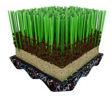
**Amorim Hybrid 301**, is a bio-based infill for high performance artificial turf systems. It is formulated with the best cork granules, virgin sbr rubber and other biodegradable materials to increase performance, even under harsh weather conditions. With size between 0.5 and 2 mm, Amorim Hybrid is a perfect match for artificial turf systems with demand for higher elasticity of infills.
