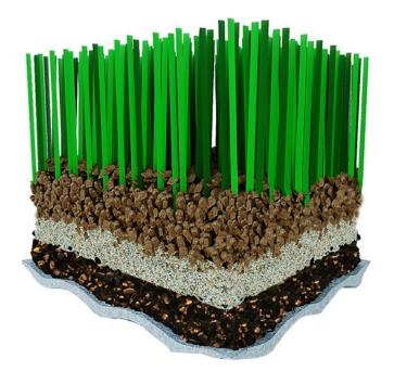
**Shockpad for artificial turf systems**, applied in situ, with a proprietary carrier mat with dimples that enables air cushioning and provides improved shock absorption. Combining rubber from recycled tires and cork provides a product that complies with FIFA requirements for shockpads.
